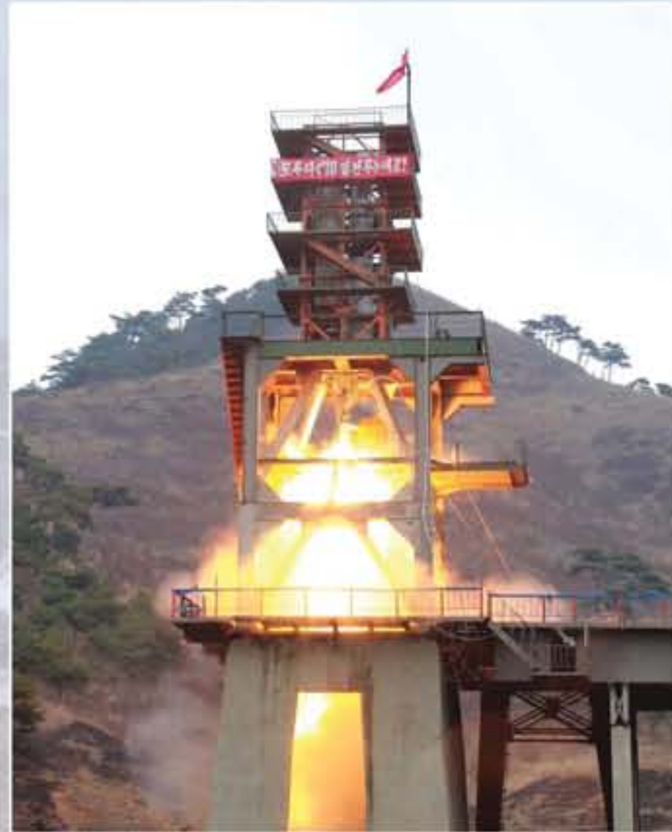
탄도로켓트 대기권재돌입환경모의시험 Re-entry simulation test of ballistic rocket
